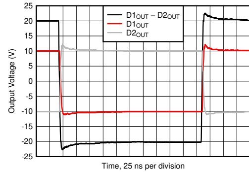
Figure 6-50. Large-Signal Pulse Response
